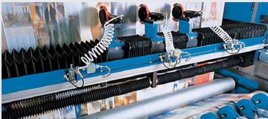
Slitters guarantee a precise scissor cut
