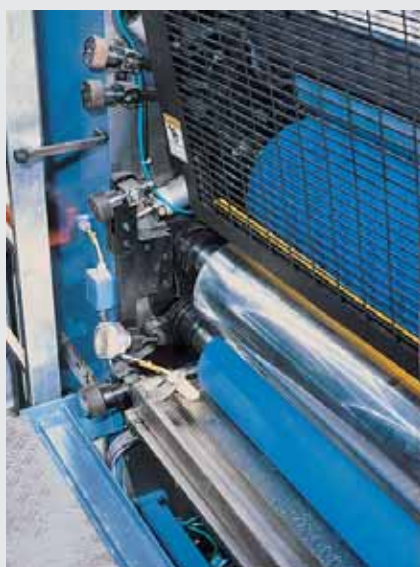
Dampening unit for alcohol-free printing
