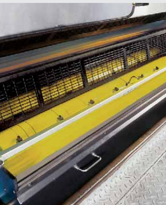
Film inking unit for a superb print quality
